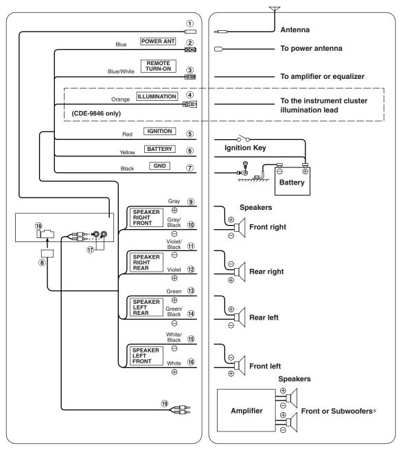
\* When Subwoofer is set to OFF: Output is from Front speakers. When Subwoofer is set to ON: Output is from Subwoofer.
